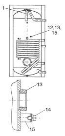
Remove screw plug (12). Apply sealing paste to the thread of the external current anode (4) before screwing in. Screw Correx external current anode (8) into the 3/4" coupling sleeve (13) using a 1/2" reduction union piece. Connect connecting cable (3) from casing (1) to the external current anode (7) using a flat plug connection.
