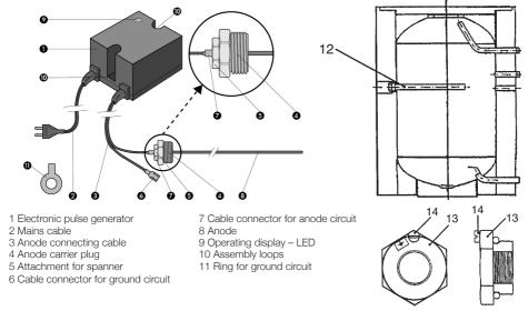
Remove magnesium anode (12). Clean thread; screw in transition piece (13) with O ring (no hemp). Apply sealing paste to the thread of the external current anode (4) before screwing in. Screw external current anode (8) into the transition piece (13). Connect connecting cable (3) from casing (1) to the external current anode (7) using plug.
